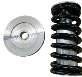
FIG. 36 - ACTUATOR PISTON "CUP" OR "BORE" WHERE SPRING ASSEMBLY FITS
