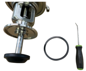
FIG. 10 - GASKET REMOVED TO BE REPLACED
